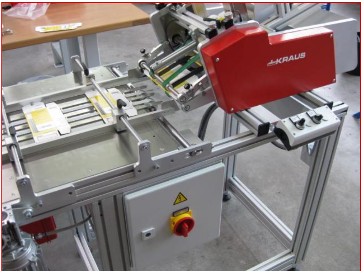
Studded conveyor system with lateral guides
