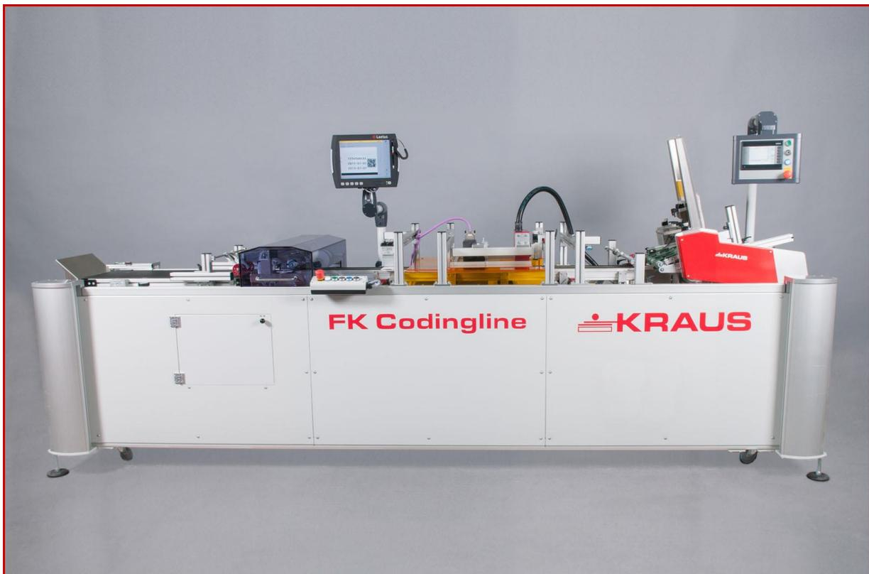
*FK Codingline consisting of: friction feeder, vacuum conveyor, rejection unit with catch box and integrated shingle outfeed conveyor*
