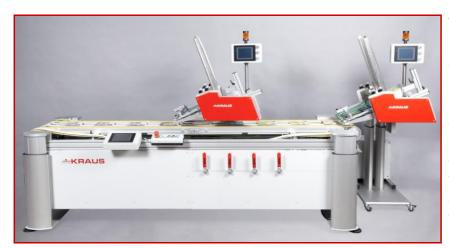
The base plate has a height of less than 90 mm allowing it to be inserted under most production lines. The frame available as an electric, height-adjustable model or as a simpler model with fixed height а adapted to the height of your conveyor machine.
