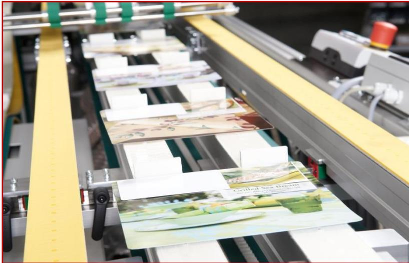
Suction tracks can be regulated and opened and closed individually with special shut-off valves. The vacuum pump is equipped with a sound suppressor. Servo friction feeders are designed as independent modules so that they can be used with various systems.
